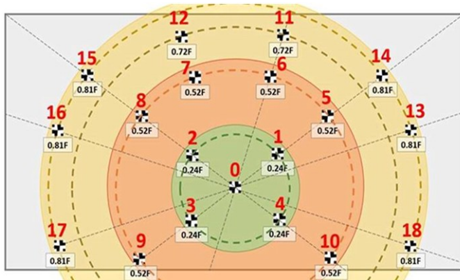
Fig. 2. Test board with slanted-edge patterns with marked detection areas of the camera image sensor
