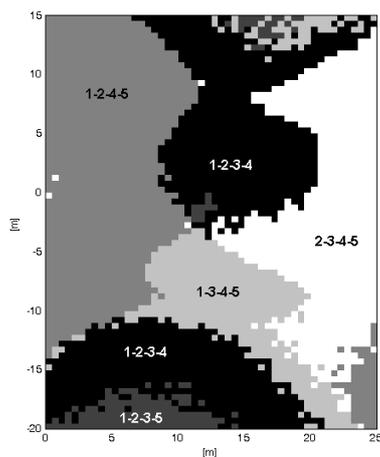
Fig. 6. Transmitter configurations providing minimum positioning uncertainty.
