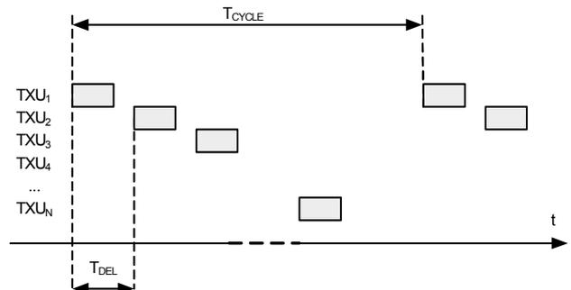
Fig. 2. Transmission pattern in a system including  $N$  TXUs.
