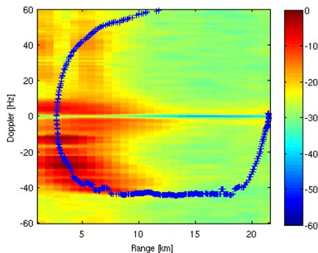
Fig. 9. Overlapping of actual flight path (Line Style '+' and colour blue) on calculated flight path (red) in compound ARD between  $-12\text{Hz}$  and  $-42\text{Hz}$  Doppler [3].
